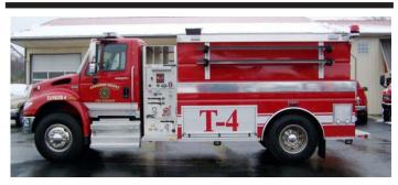
The Anderson County Fire District has taken delivery of a Wynn 500M Series Tanker. This unit features a 500-gpm Darley PTO pump, a 2000gallon Polypropylene Tank, and all LED Emergency Lighting. The apparatus body was manufactured on a 2009 International chassis by Wynn Fire Equipment, LLC.
