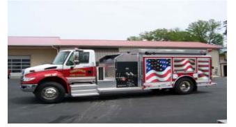
Gilbertsville Fire and Rescue has taken delivery of a Wynn 600 Series Pumper. This unit features a 1250-GPM Darley Pump Module, a 1000gallon Polypropylene Tank, and a variety of equipment. The apparatus body was manufactured on a new 2010 International chassis by Wynn Fire Equipment, LLC.
