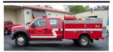
The Lincoln County Fire Protection District has taken delivery of a Wynn Brush Truck. This unit features a CET/Honda 250-gpm Pump, a 300gallon Polypropylene Tank, and a variety of equipment. The apparatus body was manufactured on a 2008 Ford chassis by Wynn Fire Equipment, LLC.
